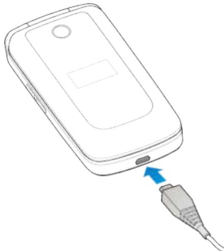
2. Connect the charger to a standard AC power outlet. If the phone is on, you'll see a charging icon, such as or , appear on the status bar.
