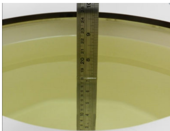
Fig 10.2 Photo of Liquid Height for Body SAR
