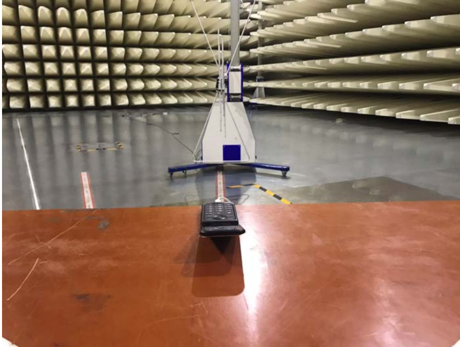
Radiated Emissions Test Setup(below 1GHz)
