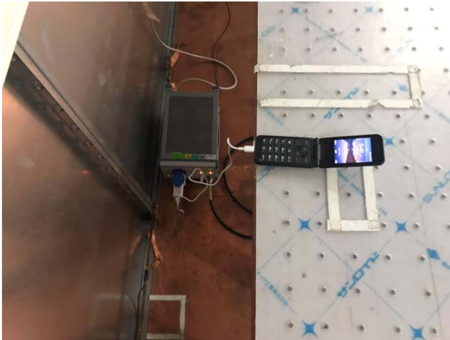
Conducted Emissions Test Setup (with charger)
