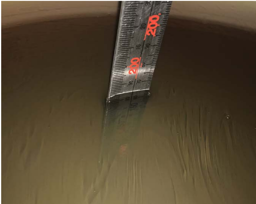
Liquid depth for SAR Measurement
