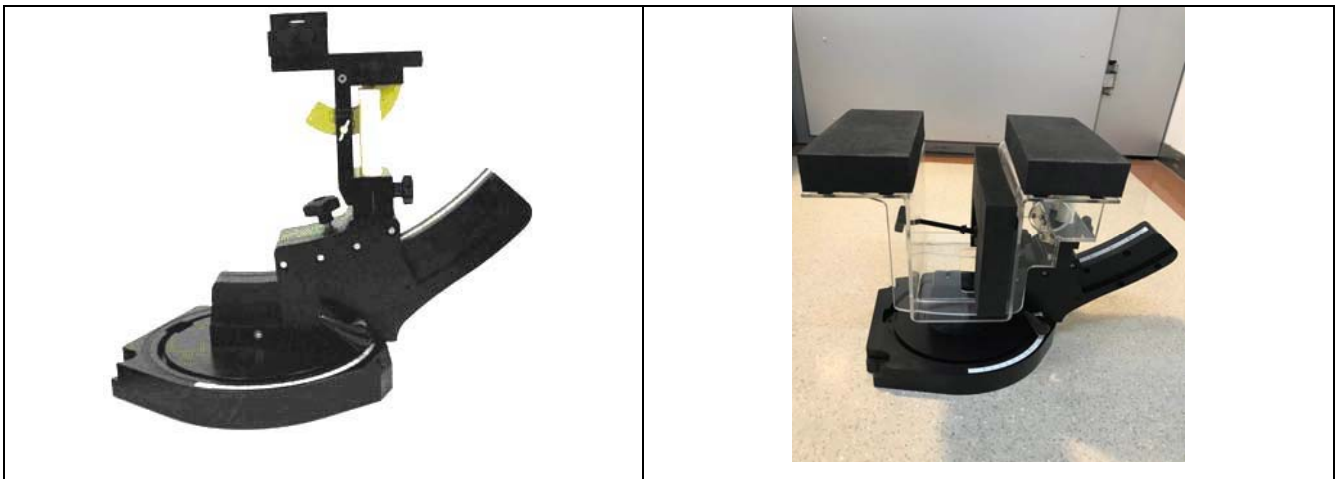
Device holder supplied by SPEAG
