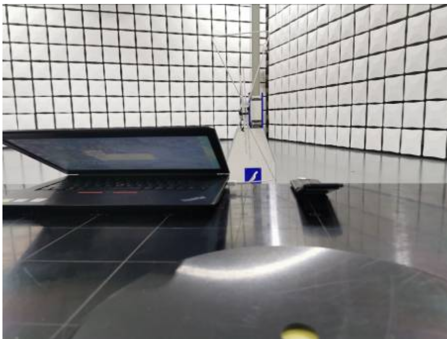
Radiated Emissions Test Setup (with laptop) (30-1000MHz)
