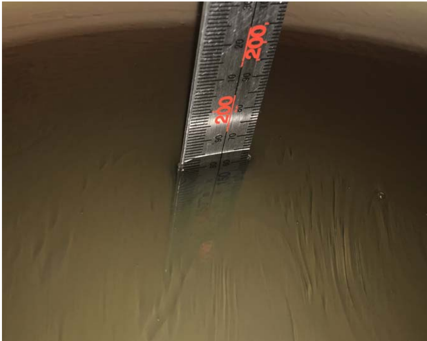
Liquid depth for SAR Measurement
