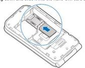
Hold your microSDHC card with the metal contacts facing down and slide it into the microSDHC card slot.
