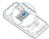
5. Insert the battery, making sure the gold contacts line up. Press down gently to secure.
