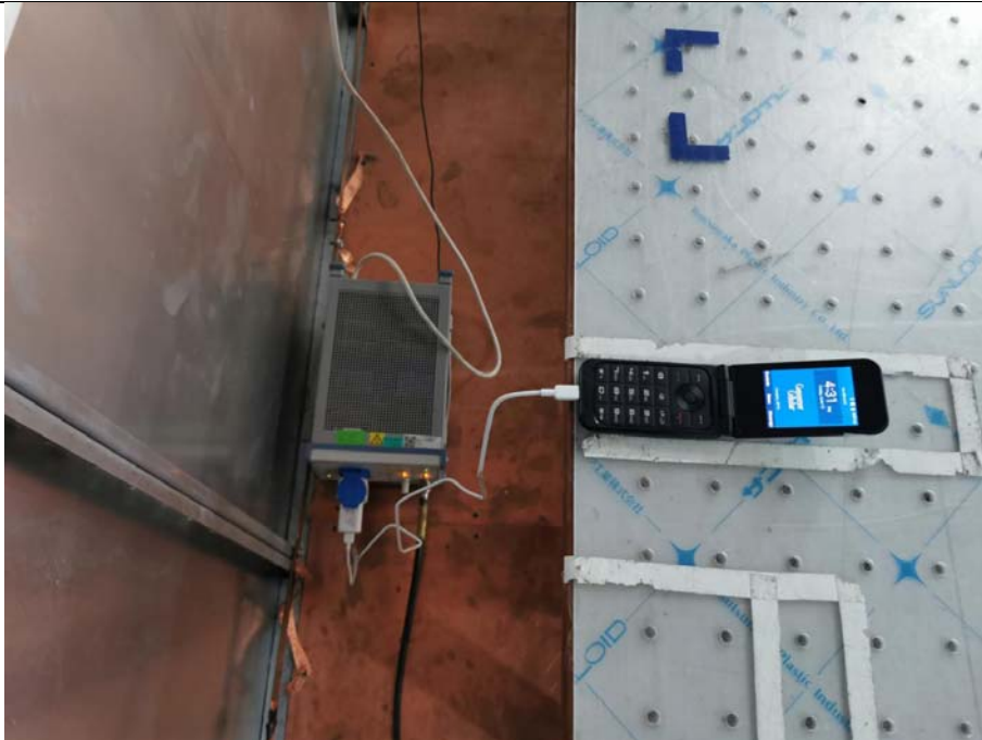
Conducted Emissions Test Setup (with charger)
