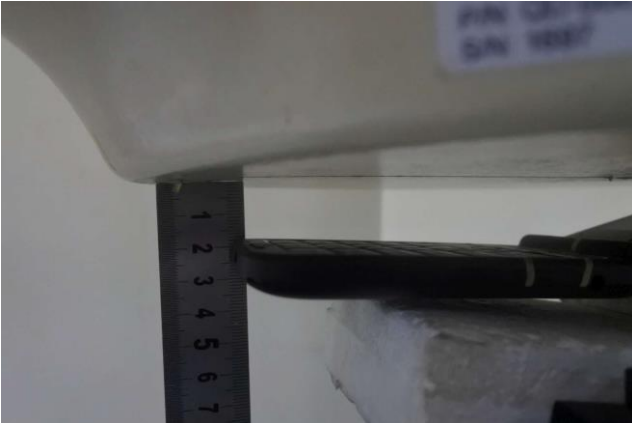
Phantom Test Separation 18 mm
