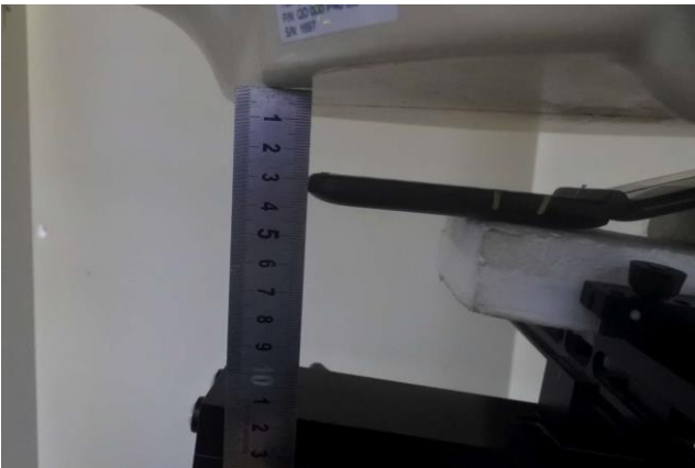
Phantom Test Separation 28 mm
