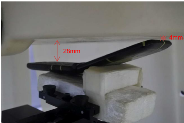
Head Test Separation 28 mm
