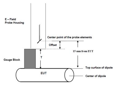
Fig. 8.3 Gauge block with E-field probe
