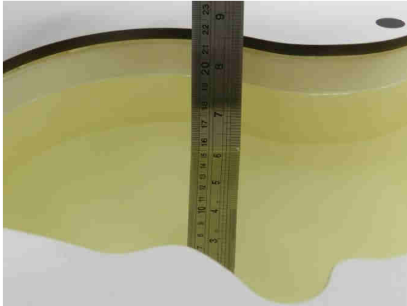
Fig 10.1 Photo of Liquid Height for Head SAR
