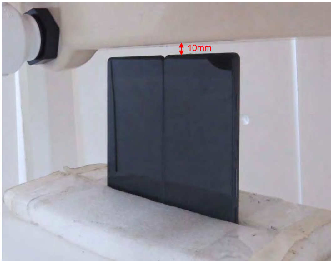
Picture 29: Bottom Side, the distance from handset to the bottom of the Phantom is 10mm For Double Screen Mode
