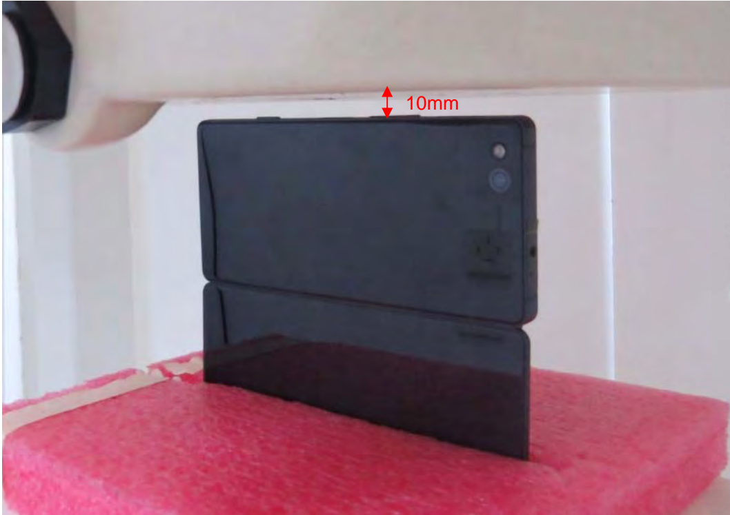
Picture 26: Left Side, the distance from handset to the bottom of the Phantom is 10mm For Double Screen Mode
