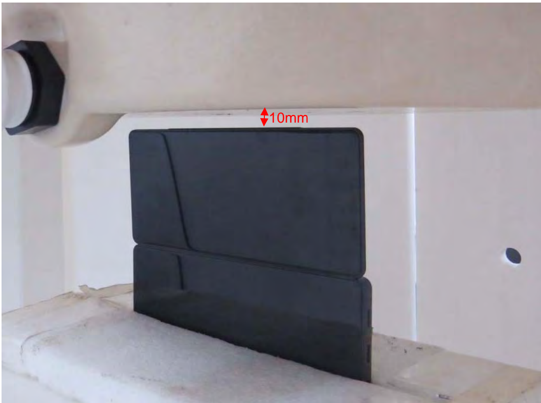
Picture 27: Right Side, the distance from handset to the bottom of the Phantom is 10mm For Double Screen Mode
