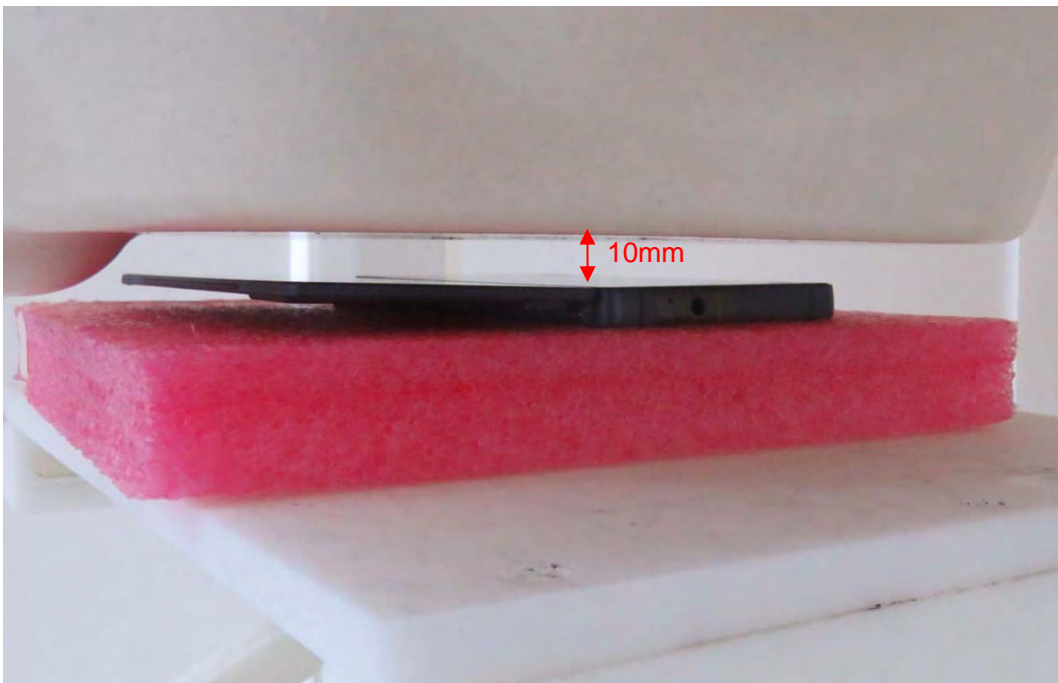
Picture 25: Front Side, the distance from handset to the bottom of the Phantom is 10mm For Double Screen Mode
