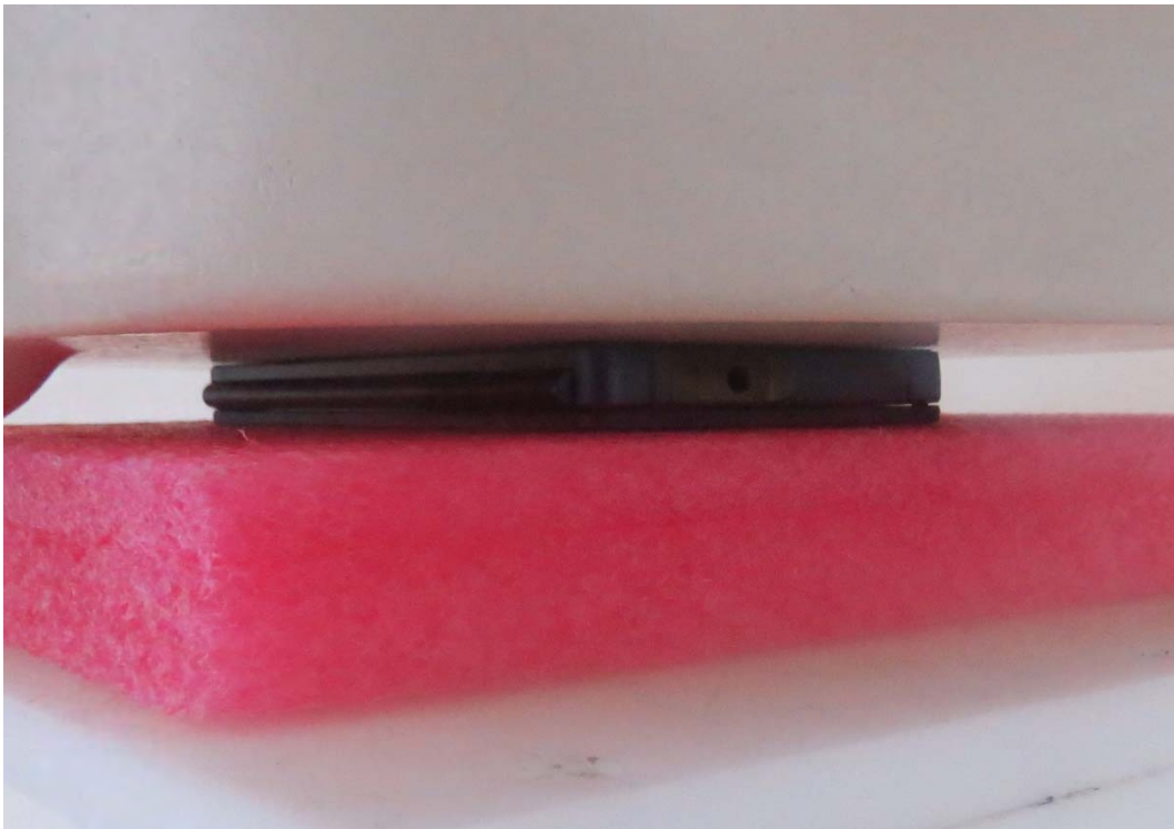
Picture 31: Front Side, the distance from handset to the bottom of the Phantom is 0mm For Single Screen Mode
