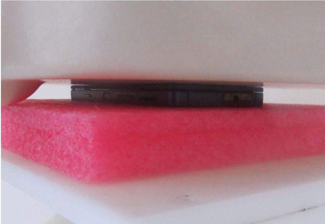
Picture 30: Back Side, the distance from handset to the bottom of the Phantom is 0mm For Single Screen Mode
