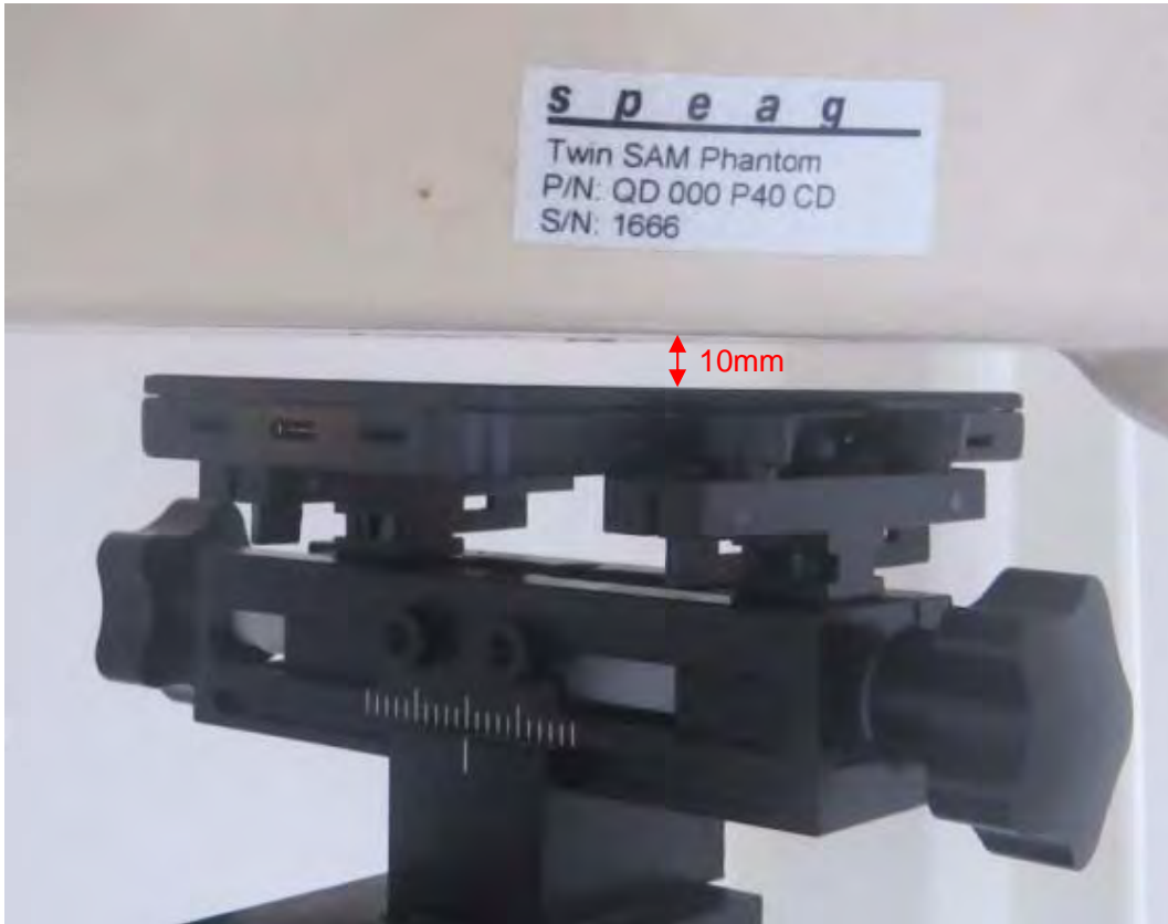
Picture 18: Back Side, the distance from handset to the bottom of the Phantom is 10mm For Single Screen Mode
