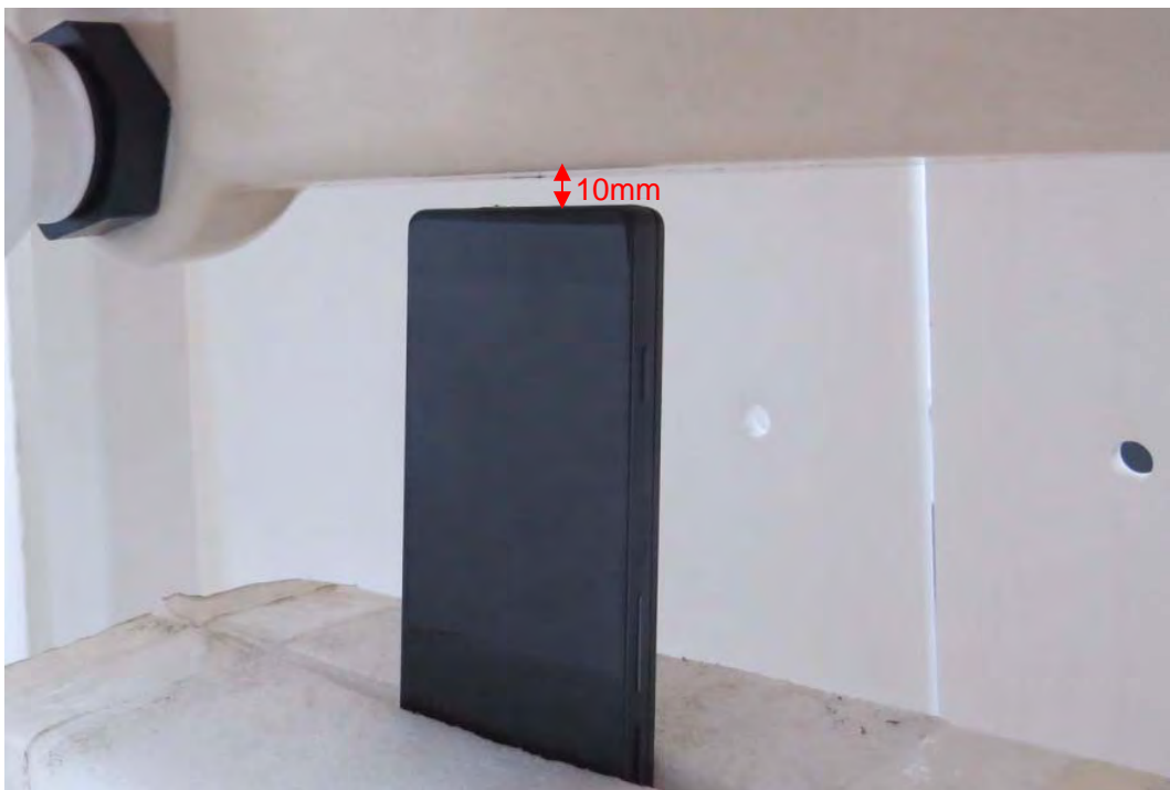
Picture 23: Bottom Side, the distance from handset to the bottom of the Phantom is 10mm For Single Screen Mode
