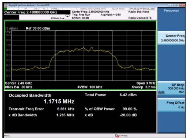
BT 2DH5 CH78, Carrier frequency (MHz): 2480
