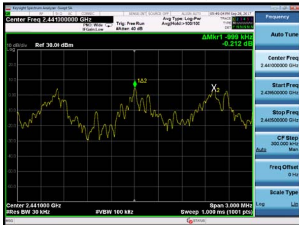
BT 3DH5 CH39, Carrier frequency (MHz): 2441
