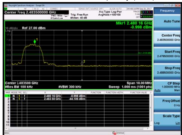
BT 3DH5 CH78, Carrier frequency (MHz): 2480
