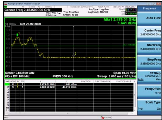
BT 2DH5 CH78, Carrier frequency (MHz): 2480
