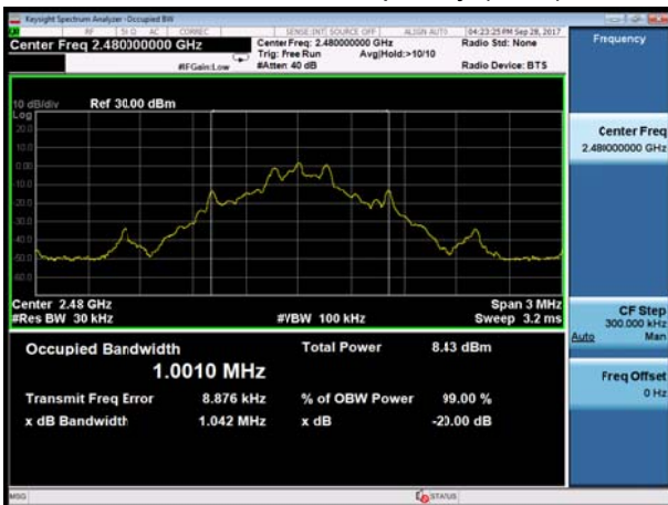
BT DH5 CH78, Carrier frequency (MHz): 2480
