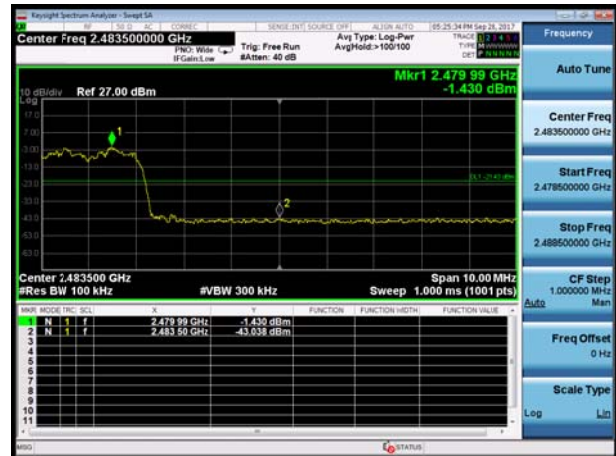
BT 3DH5 CH78, Carrier frequency (MHz): 2480
