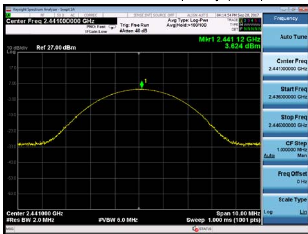
BT 3DH5 CH39, Carrier frequency (MHz): 2441
