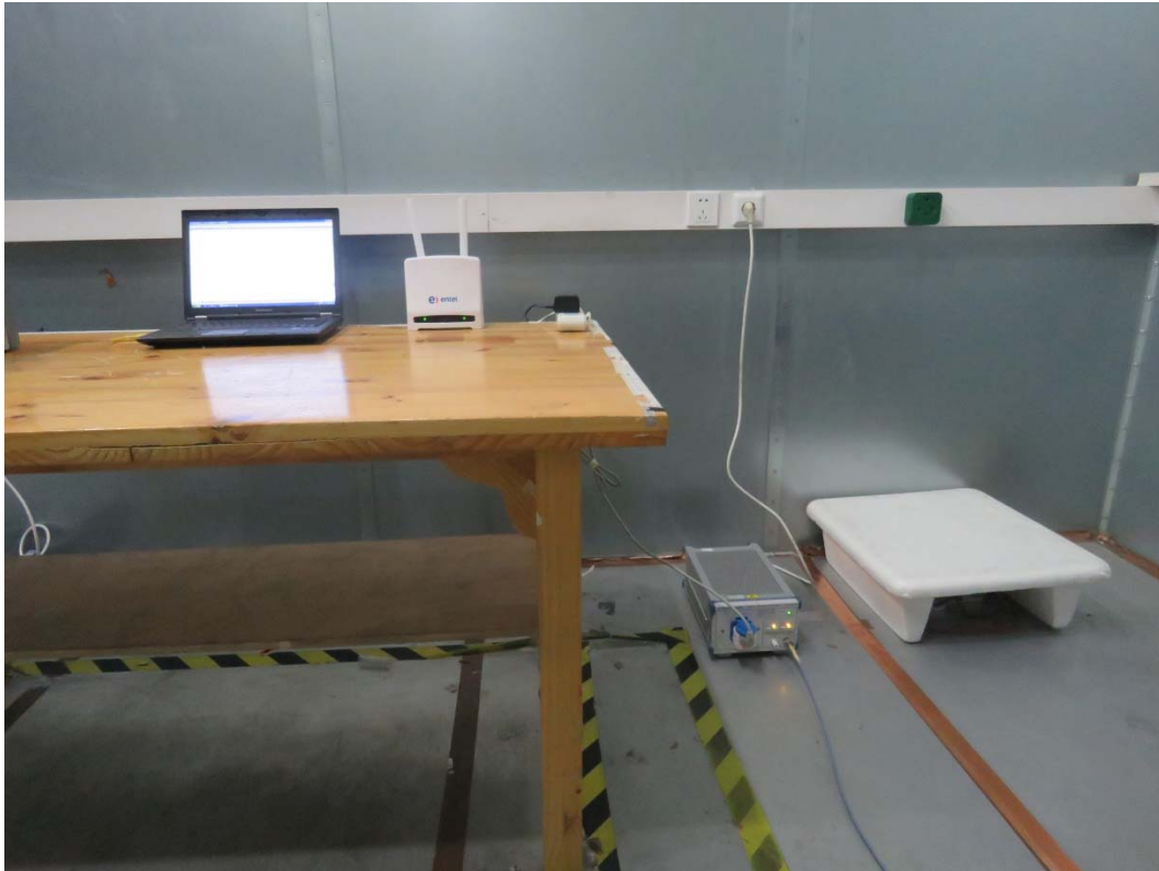
Picture 3 Conducted Emission Test Setup
