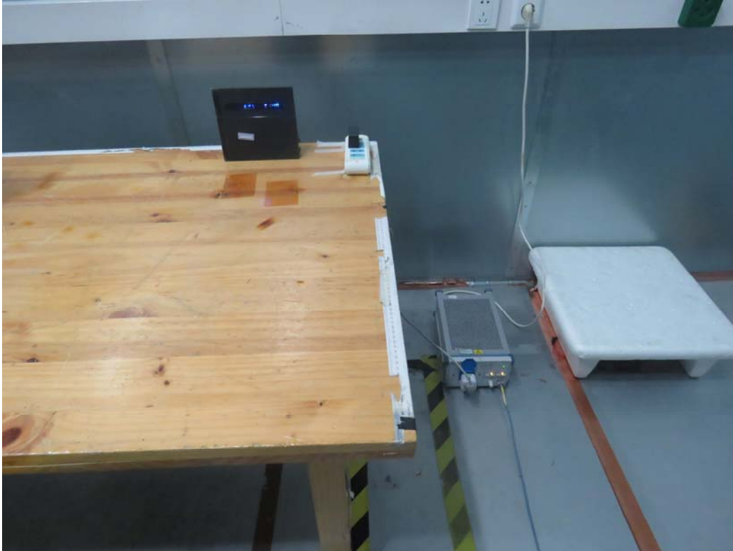
Picture 3 Conducted Emission Test Setup
