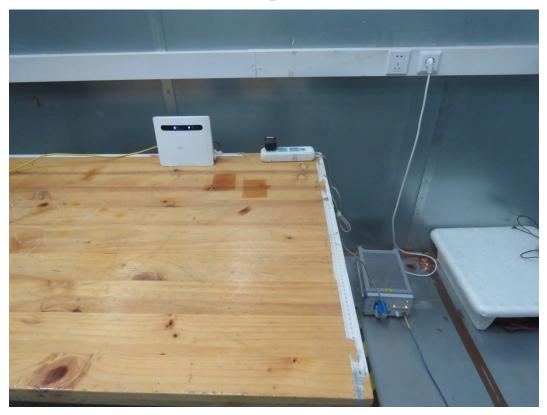
Conducted Emission Test Setup
