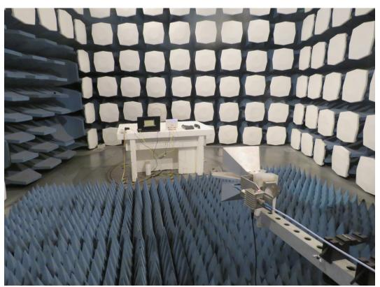
Above 1GHz Radiated Emission Test Setup
