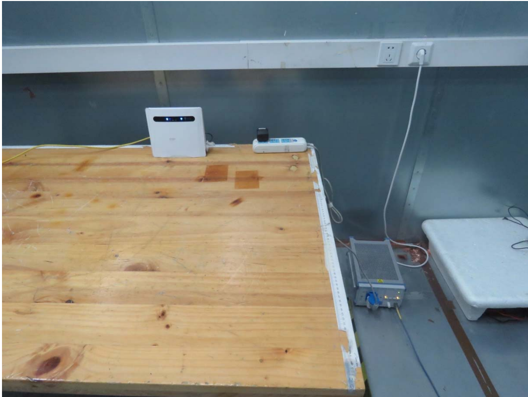
Picture 3 Conducted Emission Test Setup
