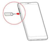
Pull out the card tray. You can place a nano-SIM card on the right card slot, and place a microSD card on the left card slot, as shown. Carefully slide the tray back into place.
