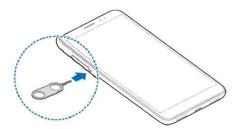
2. Pull out the card tray and place the nano-SIM card and the microSDXC card on the tray, as shown. Carefully slide the tray back into place.
