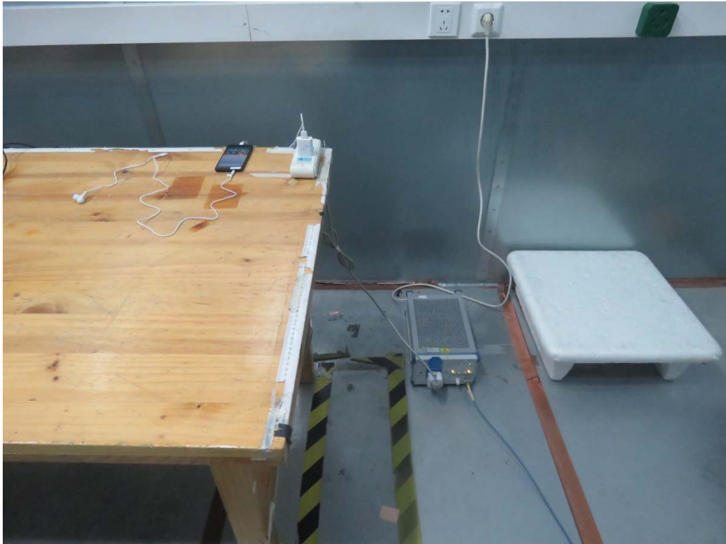
Picture 2 Conducted Emission Test Setup
