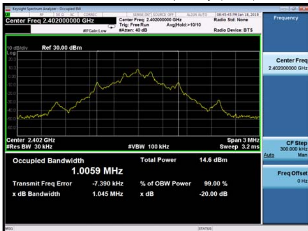
BT DH5 CH39, Carrier frequency (MHz): 2441
