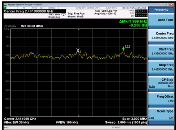
BT 2DH5 CH39, Carrier frequency (MHz): 2441
