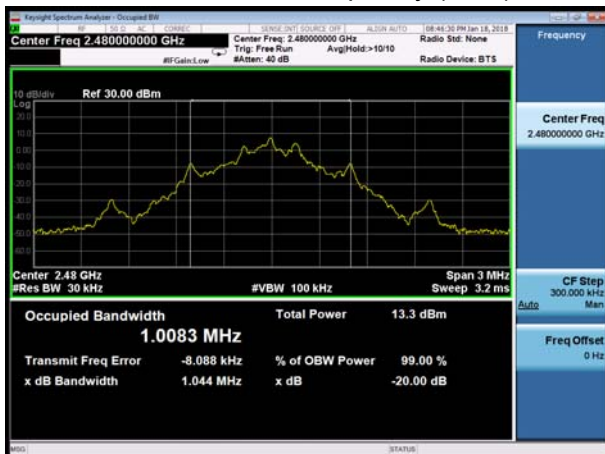
BT DH5 CH78, Carrier frequency (MHz): 2480
