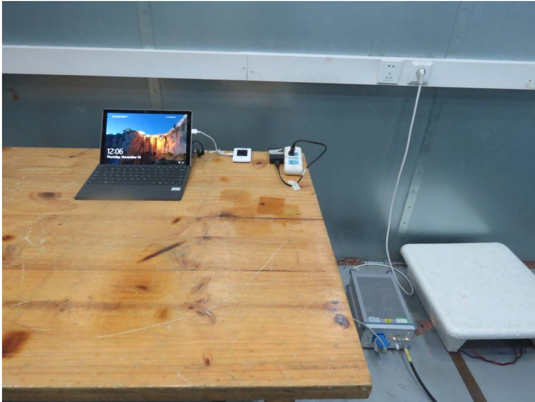
Picture 2 Conducted Emission Test Setup
