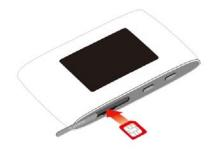
Note: usage of SIM card adapters could damage the SIM card card reader.
