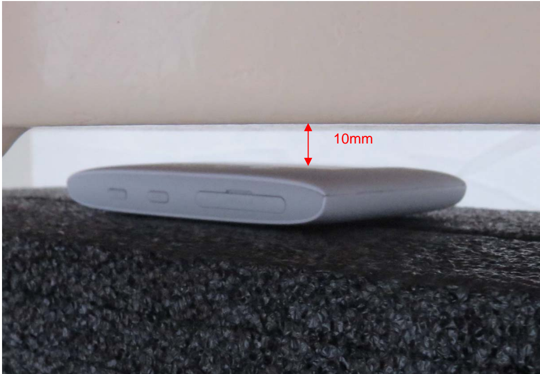
Picture 1: Back Side, the distance from handset to the bottom of the Phantom is 10mm
