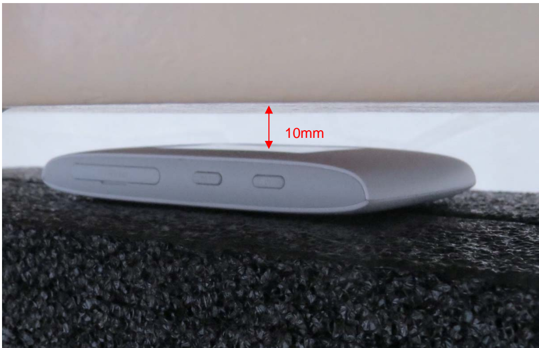
Picture 2: Front Side, the distance from handset to the bottom of the Phantom is 10mm
