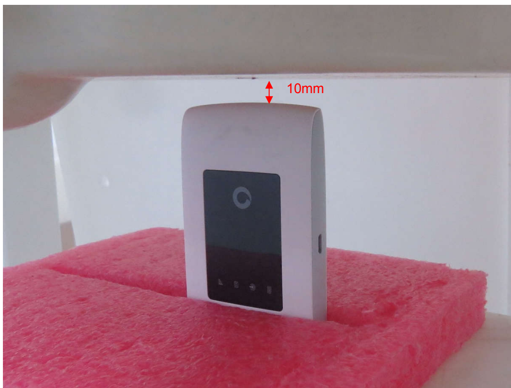
Picture 3: Left Side, the distance from handset to the bottom of the Phantom is 10mm
