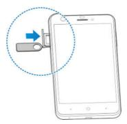
Place the microSDXC card on the tray with the gold-colored contacts facing down. Then carefully slide the tray back into place.
