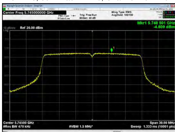
U-NII-3, 802.11ac VHT20, Channel No.: 157
