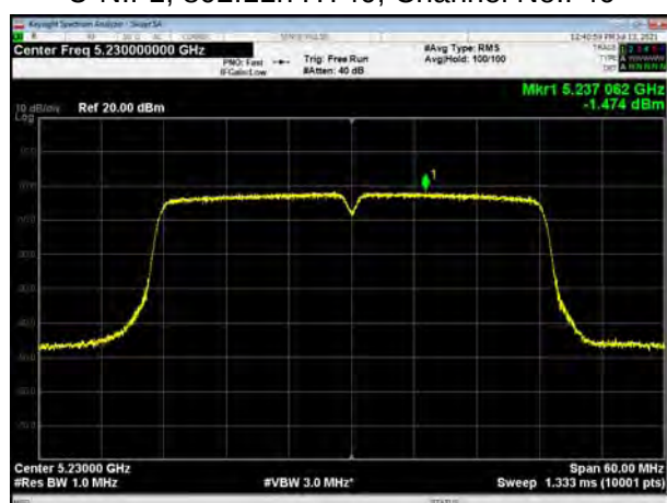
U-NII-1, 802.11ac VHT40, Channel No.: 38
