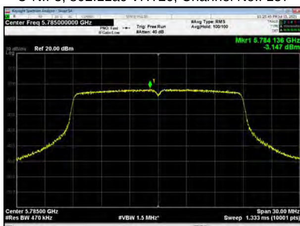
U-NII-3, 802.11ac VHT20, Channel No.: 165
