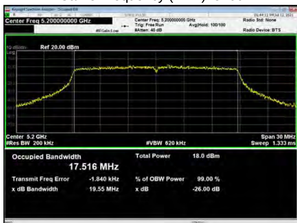
U-NII-1, 802.11n HT20 Carrier frequency (MHz): 5240
