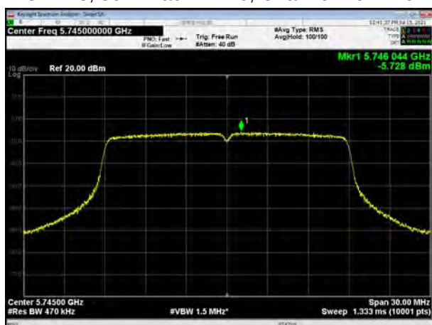
U-NII-3, 802.11ac VHT20, Channel No.: 157
