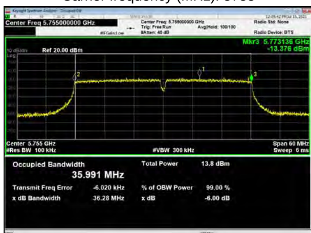
U-NII-3, 802.11ac VHT40 Carrier frequency (MHz): 5755
