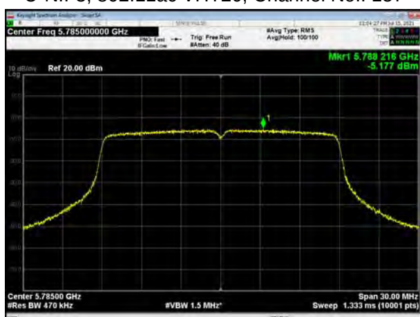
U-NII-3, 802.11ac VHT20, Channel No.: 165
