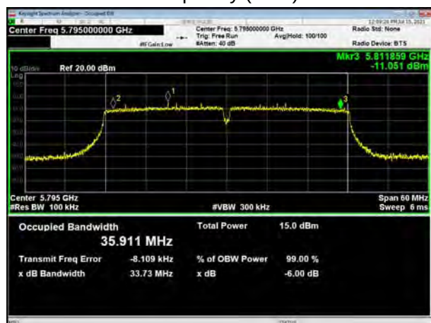
U-NII-3,802.11ax HE20 Carrier frequency (MHz): 5745
