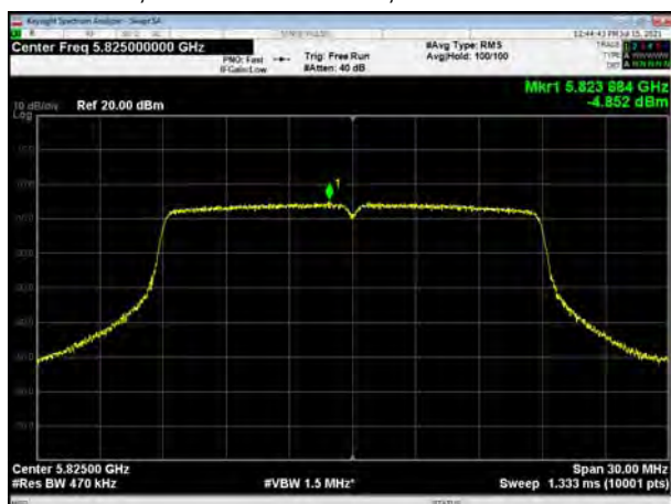
U-NII-3, 802.11ac VHT20, Channel No.: 165
