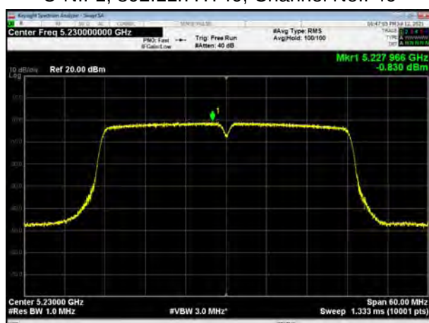
U-NII-1, 802.11ac VHT40, Channel No.: 38
