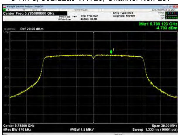
U-NII-3, 802.11ac VHT20, Channel No.: 165
