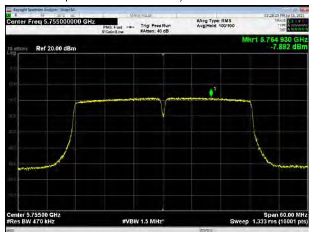
U-NII-3, 802.11ac VHT40, Channel No.: 151
