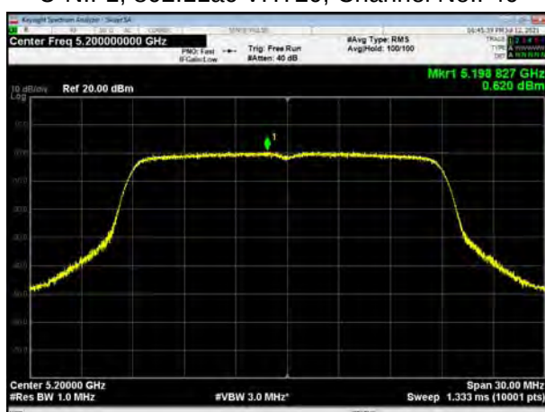
U-NII-1, 802.11ac VHT20, Channel No.: 48
