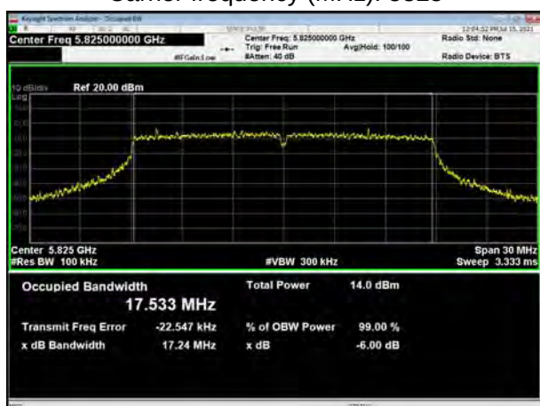
U-NII-3, 802.11ac VHT20 Carrier frequency (MHz): 5825
