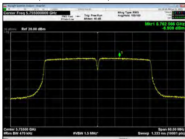
U-NII-3, 802.11ac VHT40, Channel No.: 151
