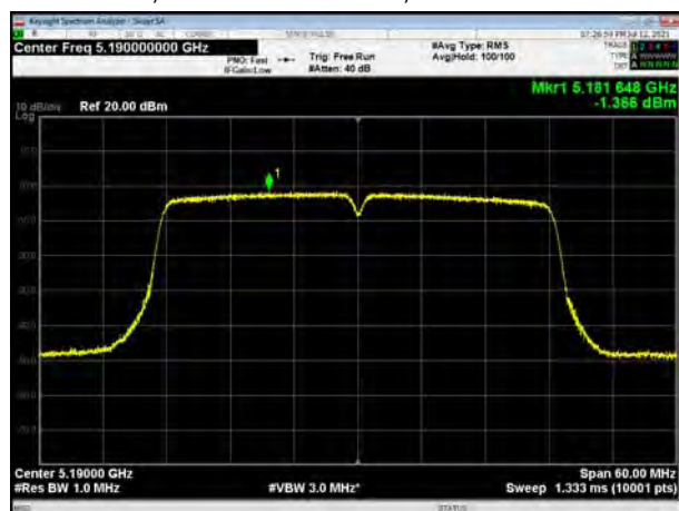
U-NII-1, 802.11ac VHT40, Channel No.: 38
