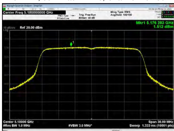
U-NII-1, 802.11ac VHT20, Channel No.: 40
