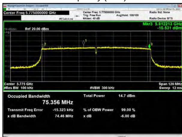
U-NII-3,802.11ax HE40 Carrier frequency (MHz): 5755
