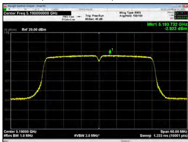
U-NII-1, 802.11ac VHT40, Channel No.: 38
