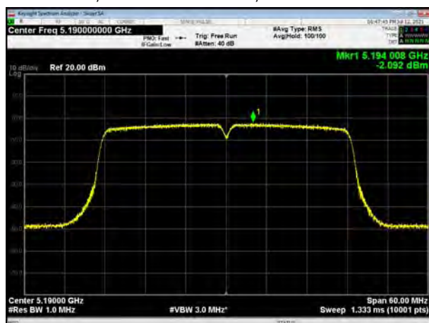
U-NII-1, 802.11ac VHT40, Channel No.: 38
