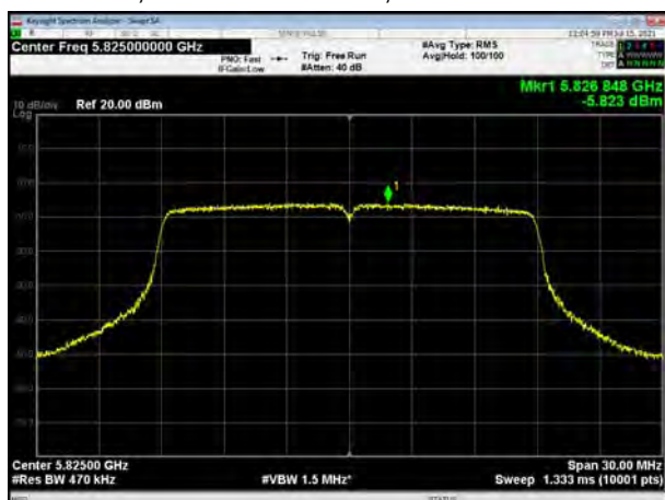
U-NII-3, 802.11ac VHT20, Channel No.: 165
