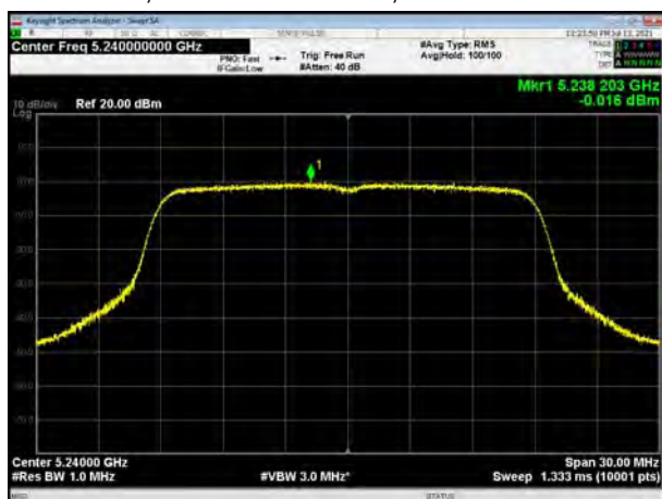
U-NII-1, 802.11ac VHT20, Channel No.: 48
