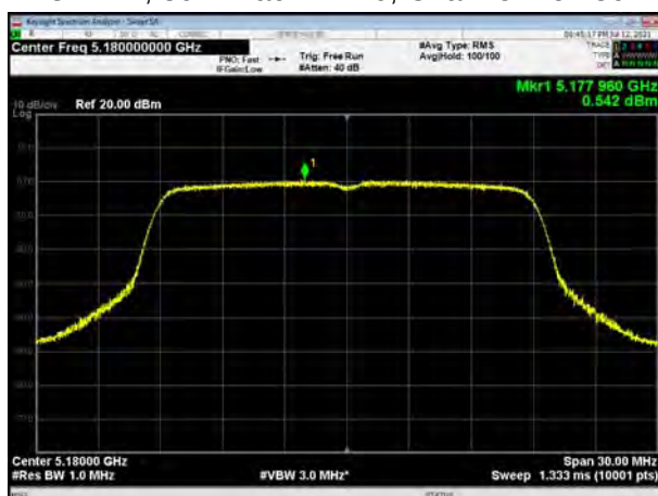
U-NII-1, 802.11ac VHT20, Channel No.: 40
