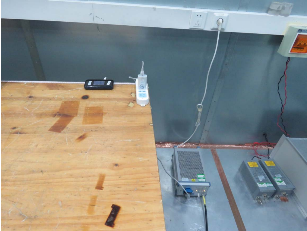
Picture 1: Conducted Emissions Test Setup
