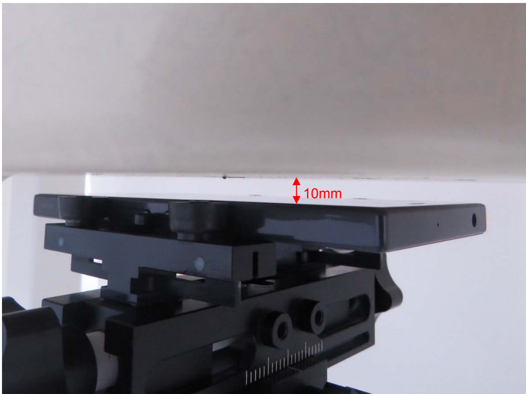
Picture 13: Front Side, the distance from handset to the bottom of the Phantom is 10mm
