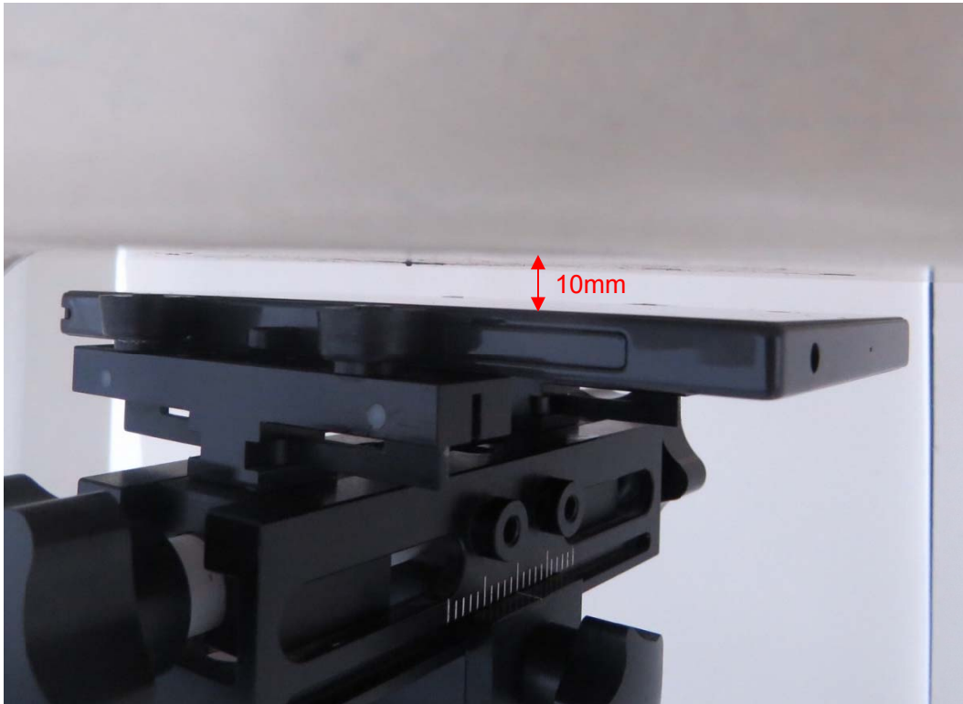
Picture 12: Back Side, the distance from handset to the bottom of the Phantom is 10mm
