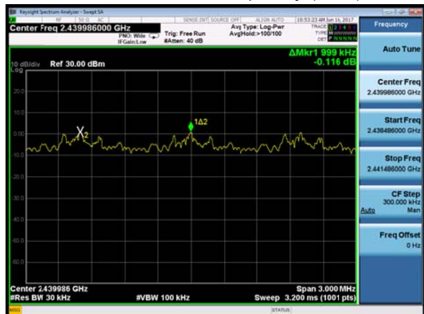
BT 2DH5 CH39, Carrier frequency (MHz): 2441
