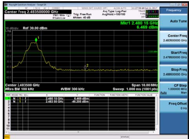
BT 2DH5 CH78, Carrier frequency (MHz): 2480
