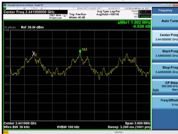
BT 3DH5 CH39, Carrier frequency (MHz): 2441
