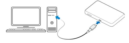
Use the adapter and the USB Type-C cable to connect an AC power outlet and your device.
