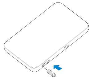
2. Pull out the card tray and place the nano-SIM card on the tray, as shown. Carefully slide the tray back into place.
