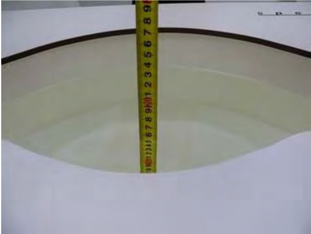
Picture 7: Liquid depth in the flat Phantom (2450 MHz, 15.3cm depth)
