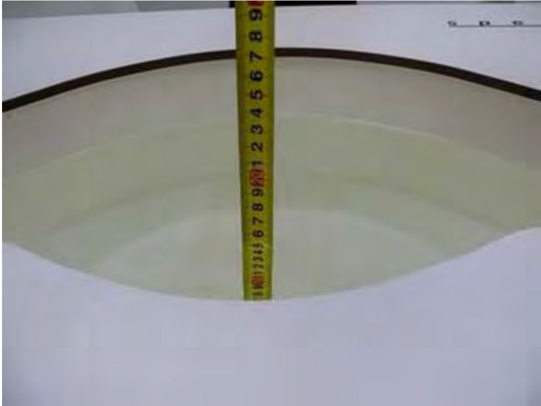
Picture 9: Liquid depth in the flat Phantom (5750 MHz, 15.0cm depth)
