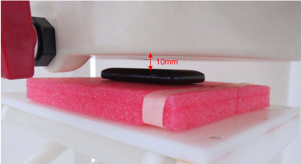
Picture 1: Back Side, the distance from handset to the bottom of the Phantom is 10mm
