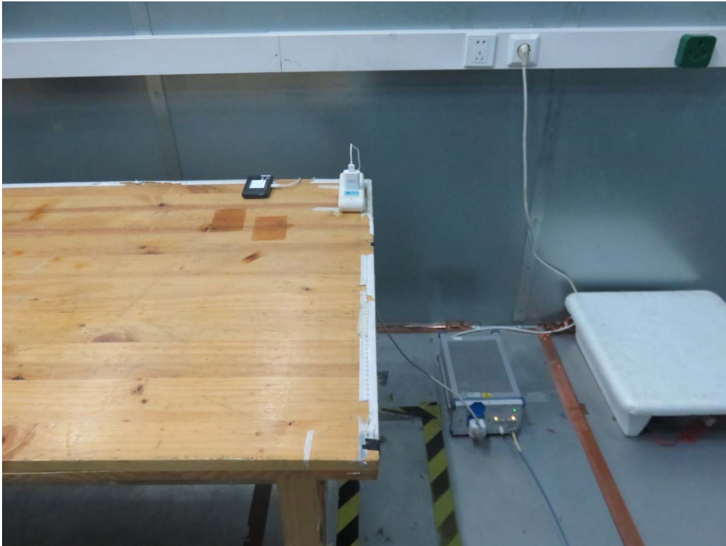
Picture 2 Conducted Emission Test Setup
