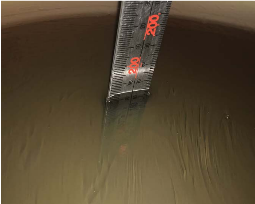
Liquid depth for SAR Measurement
