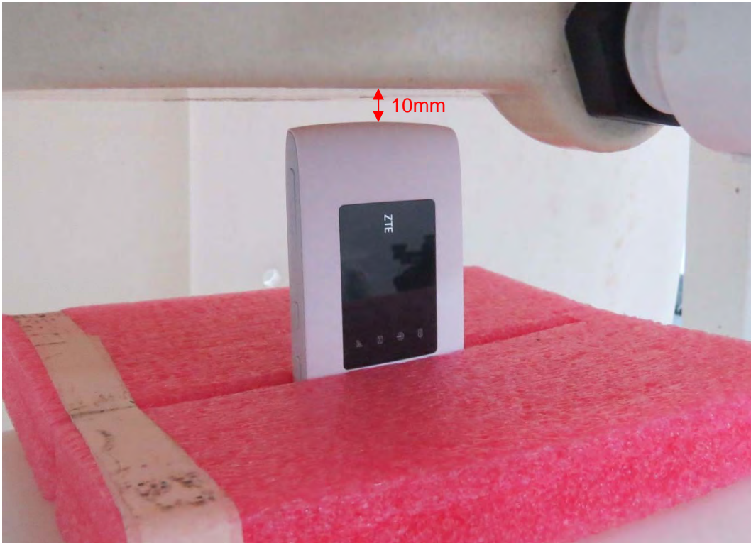
Picture 11: Left Side, the distance from handset to the bottom of the Phantom is 10mm
