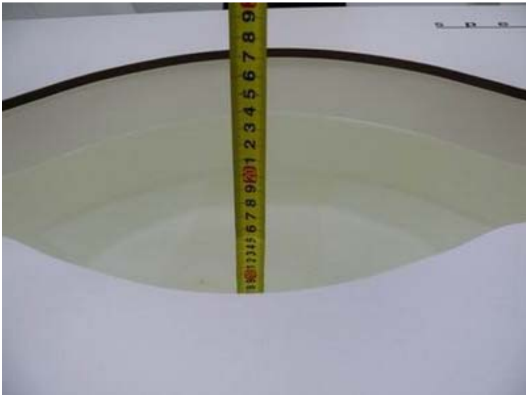
Picture 6: Liquid depth in the flat Phantom (2450 MHz, 15.3cm depth)
