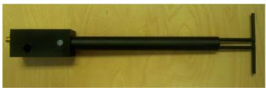
Figure 1 - MVG COMOSAR Validation Dipole
