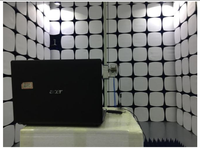
Radiated Spurious Emissions Test Setup Above 1GHz
