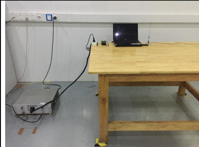
Conducted Emissions Test Setup – Front View
