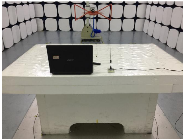
Radiated Emissions Test Setup Below 1GHz
