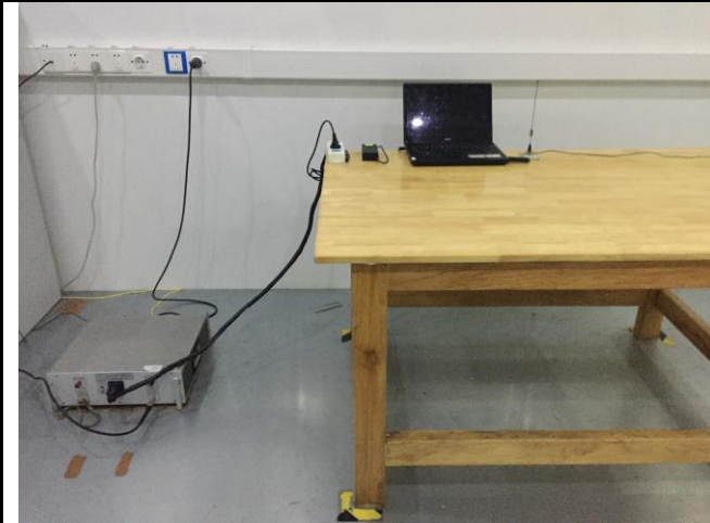
Conducted Emissions Test Setup – Front View
