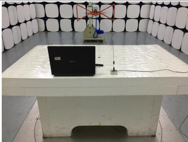
Radiated Emissions Test Setup Below 1GHz
