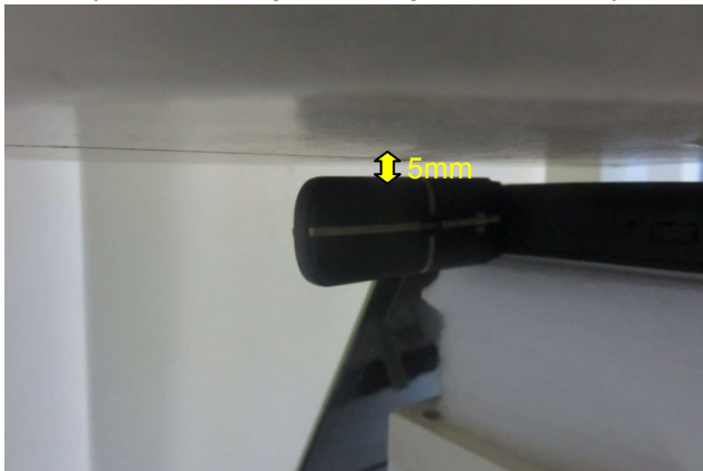
Direct Laptop Plug-in for USB Configuration 3 (Vertical Front, Test Separation 5 mm)
