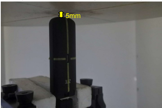
USB Cable Plug-in for USB Configuration 5 (Tip Mode, Test Separation 5 mm)
