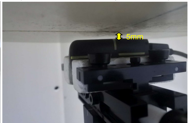
USB Cable Plug-in USB Configuration 4 (Vertical Back, Test Separation 5 mm)
