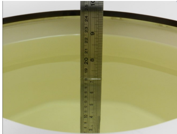
Fig 11.1 Photo of Liquid Height for Body SAR
