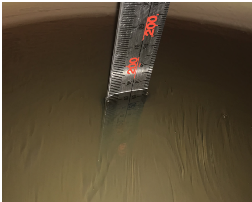
Liquid depth for SAR Measurement
