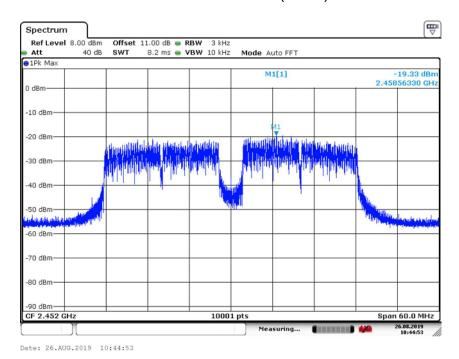
Carrier frequency (MHz): 2452 Channel No.9 Test Mode: 802.11n (HT40)
