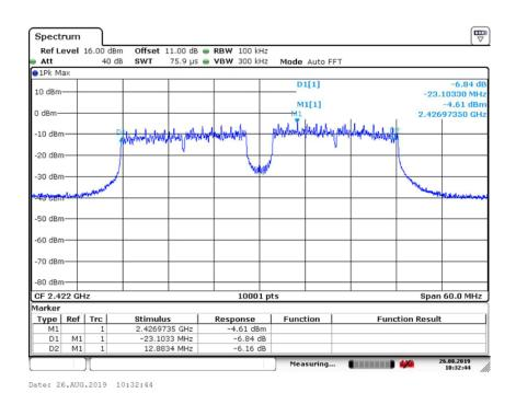
Carrier frequency (MHz): 2422 Channel No.:3 Test Mode: 802.11n (HT40)
