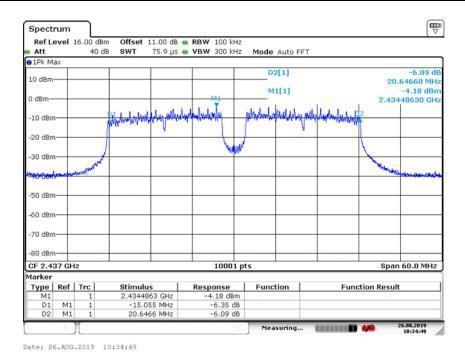
Carrier frequency (MHz): 2437 Channel No.:6
