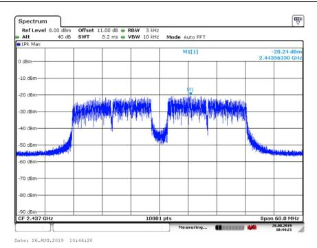
Carrier frequency (MHz): 2437 Channel No.6 Test Mode: 802.11n (HT40)
