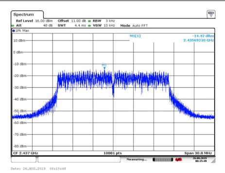
Carrier frequency (MHz): 2437 Channel No.6 Test Mode: 802.11n (HT20)
