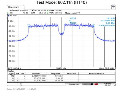
Carrier frequency (MHz): 2452 Channel No.:9 Test Mode: 802.11n (HT40)
