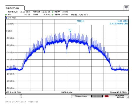
Carrier frequency (MHz): 2412 Channel No.1 Test Mode: 802.11b
