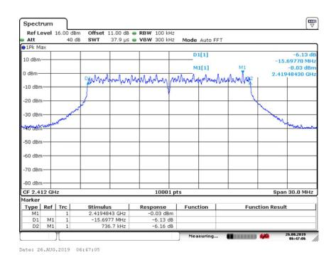
Carrier frequency (MHz): 2412 Channel No.:1 Test Mode: 802.11n (HT20)
