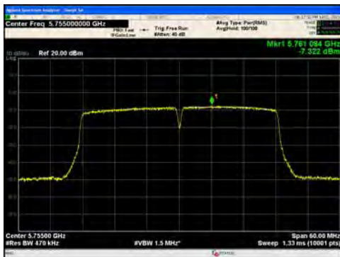
U-NII-3, 802.11ac VHT40, Channel No.: 159
