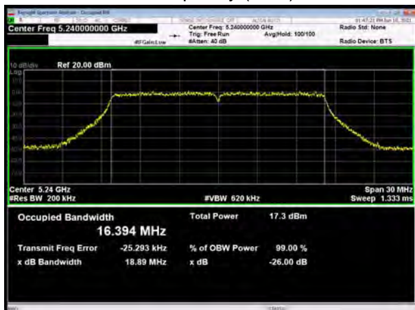
U-NII-1, 802.11a Carrier frequency (MHz):5240
