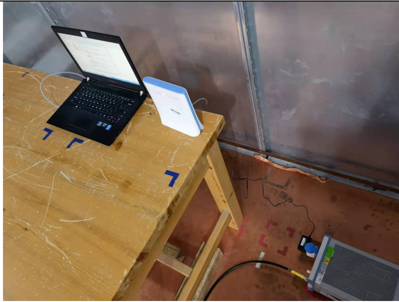
Conducted Emissions Test Setup (with charger)
