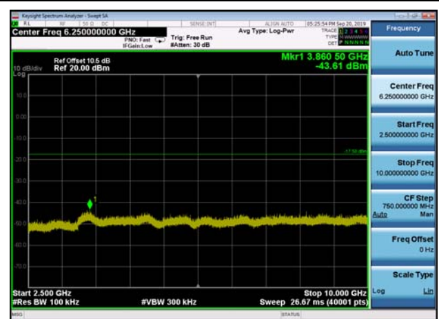
,Plot 4,2500MHz~10000MHz-802.11n(HT40 ) ,2452MHz,Ant1
