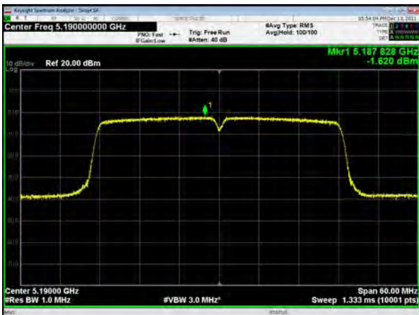
U-NII-1, 802.11ac VHT40, Channel No.: 46
