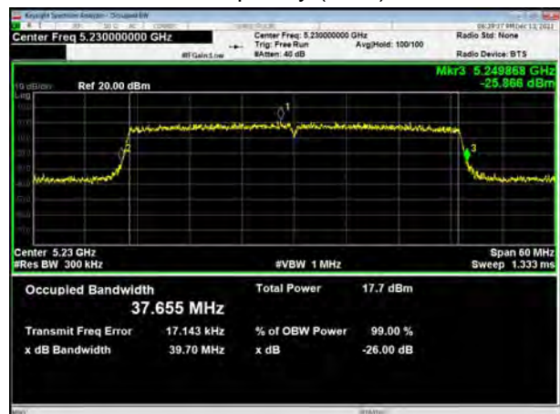
U-NII-1, 802.11ax HE40 Carrier frequency (MHz): 5230
