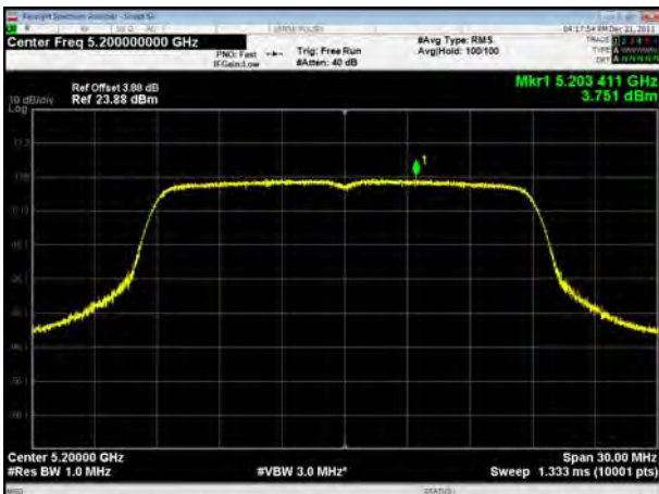
U-NII-1, 802.11ac VHT20, Channel No.: 40
