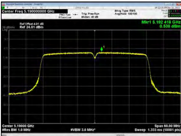
U-NII-1, 802.11ac VHT40, Channel No.: 46
