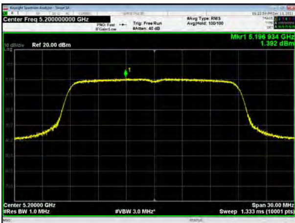
U-NII-1, 802.11ac VHT20, Channel No.: 40
