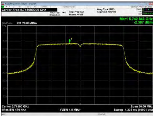
U-NII-3, 802.11ac VHT20, Channel No.: 157
