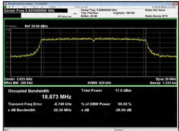
U-NII-3, 802.11ax HE40 Carrier frequency (MHz): 5755
