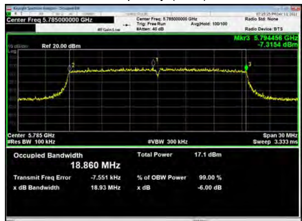
U-NII-3, 802.11ax HE20 Carrier frequency (MHz): 5785
