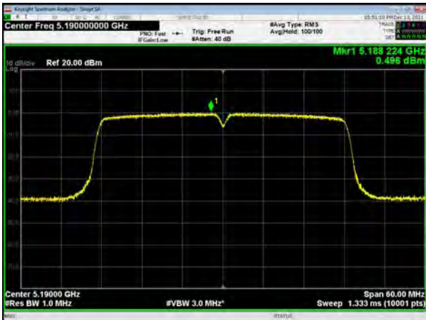
U-NII-1, 802.11ac VHT20, Channel No.: 36
