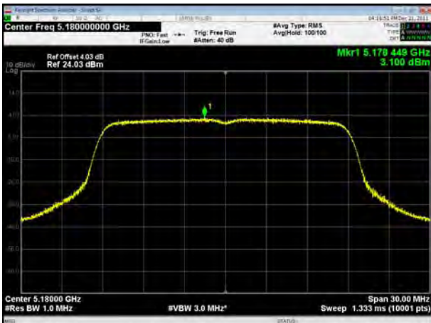
U-NII-1, 802.11ac VHT20, Channel No.: 40
