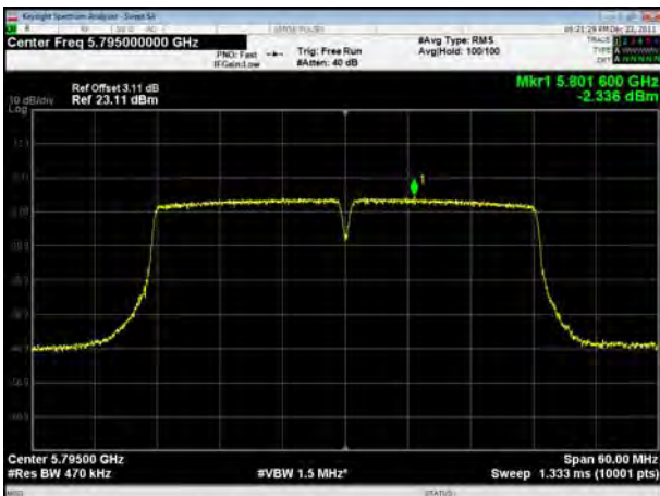
U-NII-3, 802.11ac VHT40, Channel No.: 159
