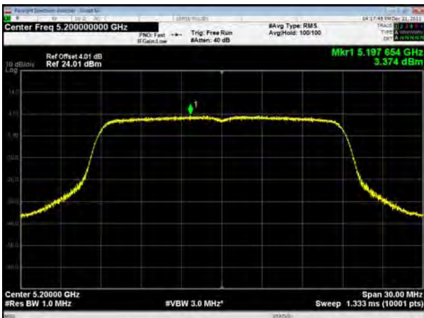
U-NII-1, 802.11ac VHT20, Channel No.: 40
