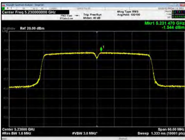
U-NII-1, 802.11ac VHT40, Channel No.: 46
