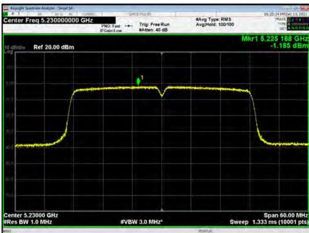
U-NII-1, 802.11ac VHT40, Channel No.: 46
