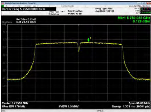
U-NII-3, 802.11ac VHT20, Channel No.: 149
