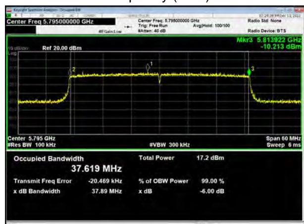
U-NII-3, 802.11ax HE40 Carrier frequency (MHz): 5795
