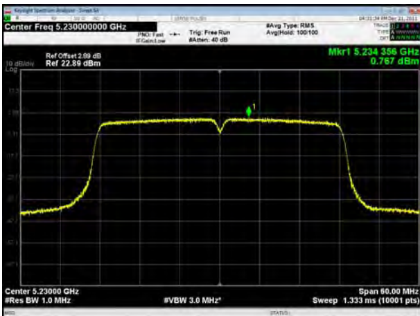
U-NII-1, 802.11ac VHT40, Channel No.: 46
