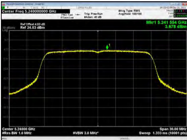
U-NII-1, 802.11ac VHT40, Channel No.: 38
