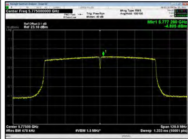
U-NII-3, 802.11ac VHT80, Channel No.: 155
