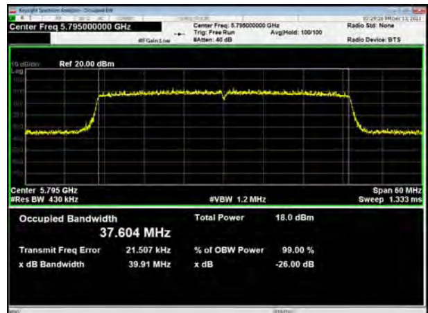
U-NII-3, 802.11ax HE40 Carrier frequency (MHz): 5795
